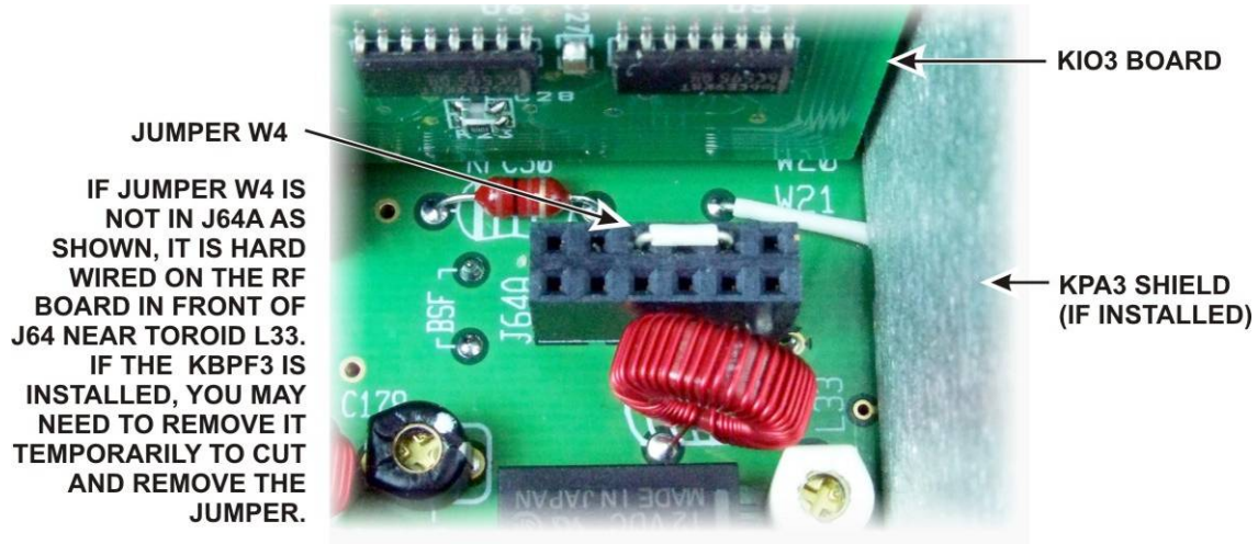
Figure 44. Jumper W4 on the K3 RF Board.
